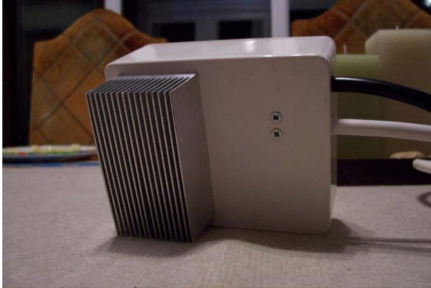
A picture from the bottom showing the heatsink. It may be a little overkill – but it is what was available in the lab at work! Having said that, the Triac does drop a few volts and with 13A going through it, the fact its encapsulated in a box, it will get hot. Adequate cooling is necessary. Even with this heatsink, I saw temperatures of 65 degrees C on the Triac body after 10-15mins. (The Triac is good for upto 120 degrees).
