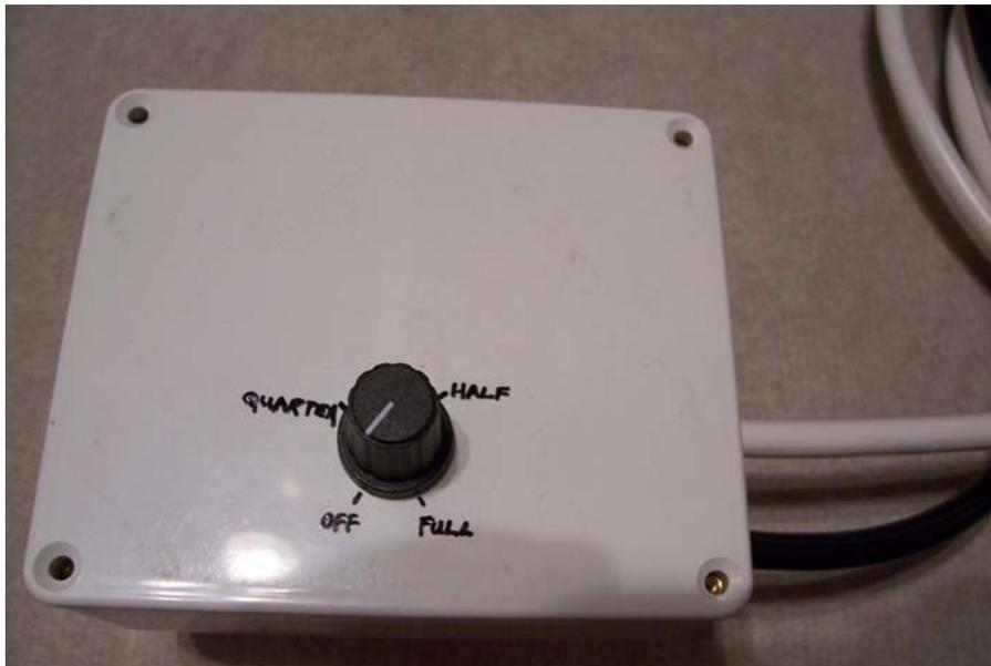
Heres the finished box. I used a current clamp and oscilloscope to work out the positions of  $\frac{1}{4}$  and  $\frac{1}{2}$  setpoints etc. I also trimmed the setpoint with the internal 1M pot. Using this you can ensure that when the main control pot is turned fully to the left – that it is actually OFF and to the right it is actually fully ON etc.
